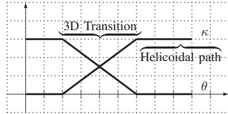
Fig. 9 Diagram of curvature  $\kappa$  and remaining climb angle  $\theta$  distributions for the three-dimensional spiral transition
