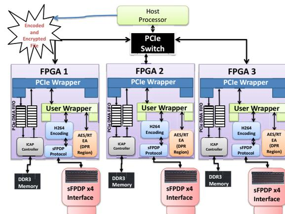
Fig. 1: Scalable distributed secure H.264 encoding on a multi-FPGA system
